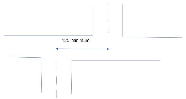
502.3 All streets shall intersect at 90 degrees whenever possible for a minimum distance of 100 feet; however, in no instance shall they intersect at less than 80 degrees onto Arterial or Collector streets or less than 50 degrees on to local streets
