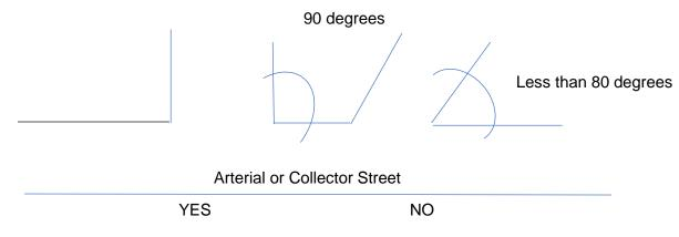
502.4 To ensure adequate sight distance, when the street centerlines deflect more than 10 degrees, connections shall be made by horizontal curves. The minimum centerline radius for local residential streets shall be 150 feet and for all other residential streets shall be 300 feet.
