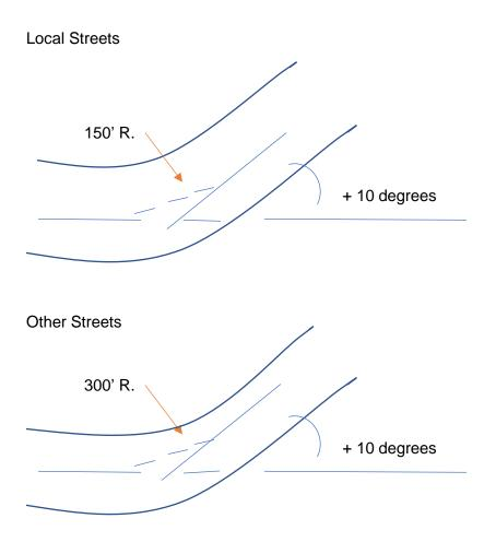
502.5 A tangent of at least 100 feet shall be introduced between reversed curves on local and collector streets.
